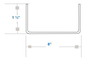
This structural framing member is designed to be placed on top and bottom to secure wall studs to form a lightweight structure. It serves to form roof truss assemblies, loadbearing walls, curtain walls and joists.
